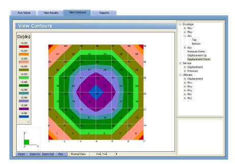
When concrete punching shear capacity is exceeded, a message box will appear during the solution indicating that concrete punching shear capacity exceeded. However, the solution will complete and results and contour views will be generated. When the user wants to display ultimate-level punching shear results, the report will display the status of the failed column and/or pile as unsafe, shown here:
