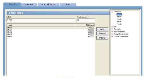
Alternatively, you can click on the Define button located on the toolbar, and then on the PROPERTIES tab.
