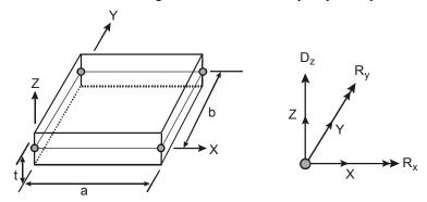
Figure 2-4 Plate Finite Element
