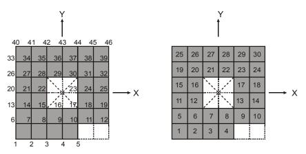
Figure 2-3 Node and Element Numbering
