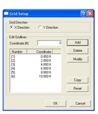
Note: As grid lines are added, new elements may be generated automatically which increases the size of the model. In order to solve large models on systems with limited memory resources<sup>34</sup>, the user may need to delete some grid lines or elements later to ensure that the model can be solved within the currently available memory.
