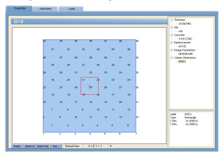
To facilitate assignment of columns, options to show the element and node labels are provided in the pop-up menu accessible by right-clicking on any blank portion of the GRAPHICS/INPUT AREA.
