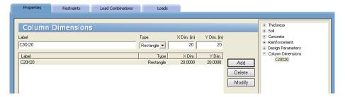
• Enter a label or Column ID in the LABEL text box and select the TYPE of COLUMN (Round or Rectangle) from the drop-down list.
