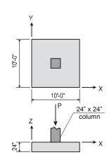
The origin of the XY plane will be located at the lower left-hand corner of the footing. Two-foot square elements will be used; thus, the grid system consists of six grid lines (i.e. five elements), two feet apart, in each direction. The concentrated load will be applied as four nodal loads (125 kip each). The finite element mesh is shown at the end of this example.
