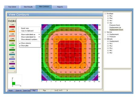
If columns have been assigned to the model, they are displayed to scale in black color. If piles have been assigned to the model, they are displayed to scale in dark red color. To not show columns or piles, right-click on empty space on the view window, and then uncheck Show Columns or Show Piles on the pop-up menu.
